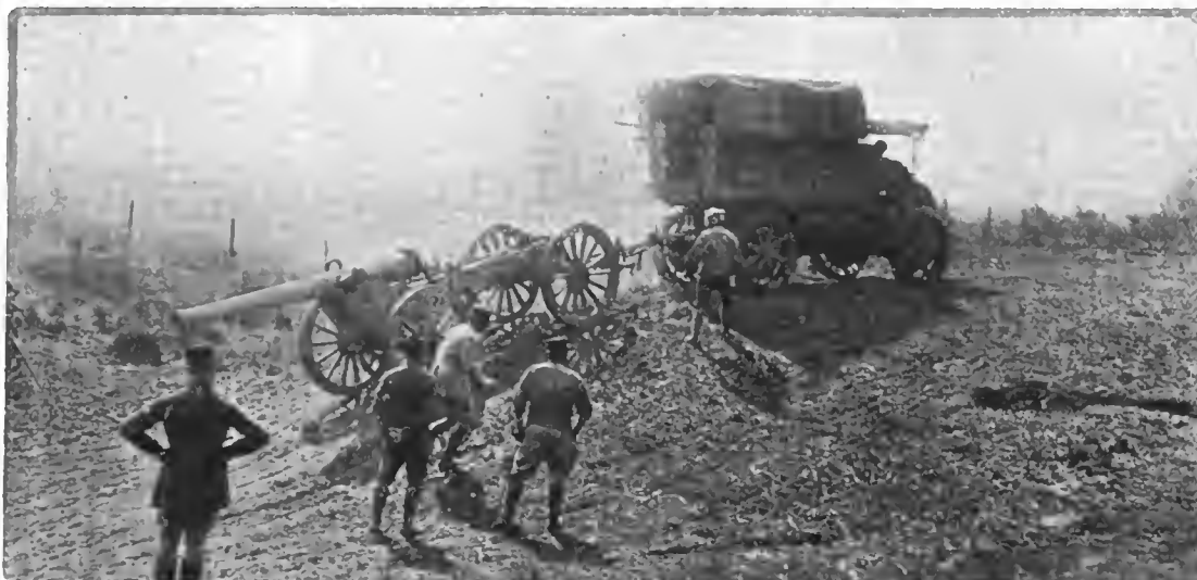
Renault tractor near the front pulling a heavy field piece up a steep incline
